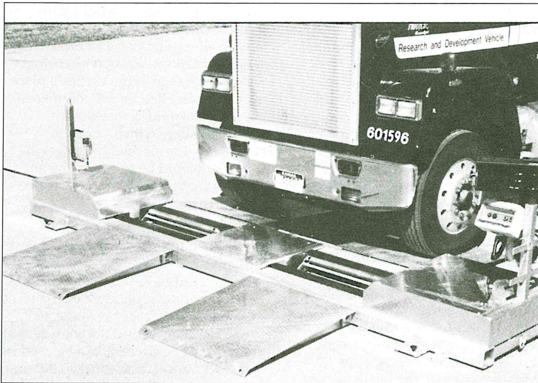
Computerized roller dynamometer brake testing equipment
