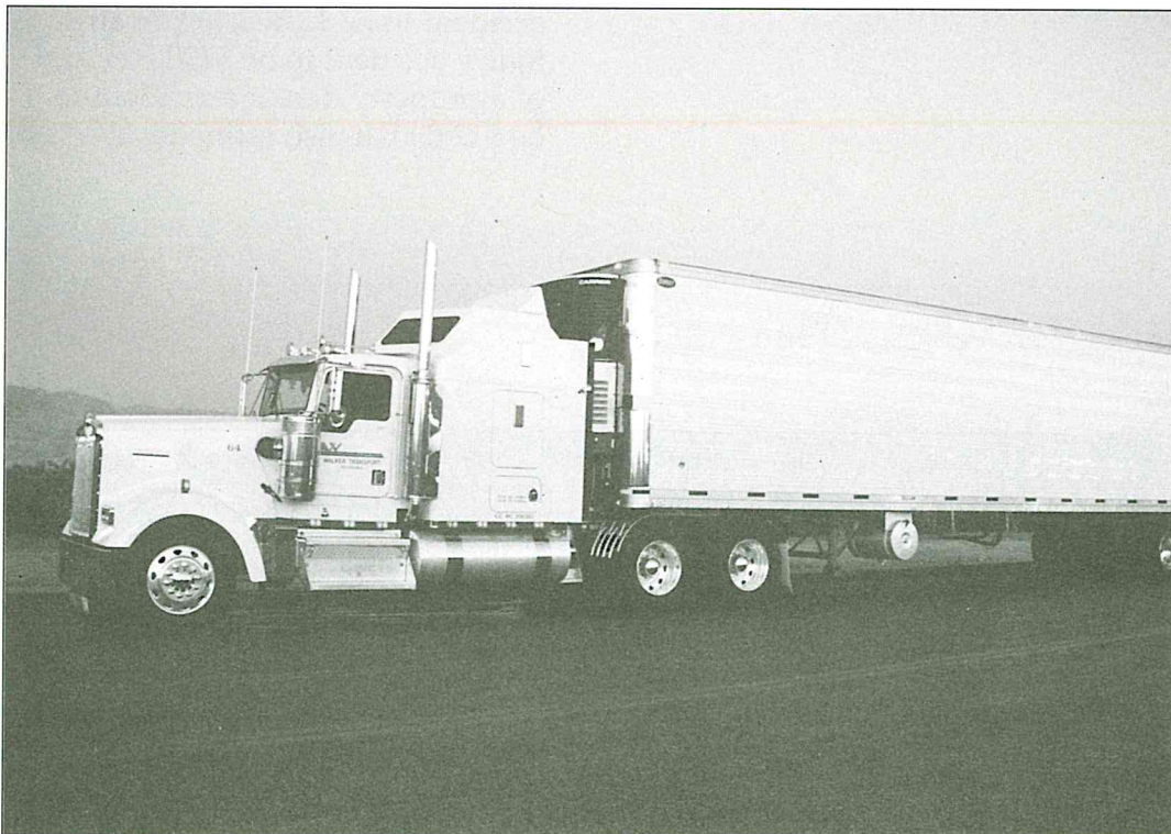
Typical tractor-trailer unit with gross vehicle weight of 39,500 kgs.
